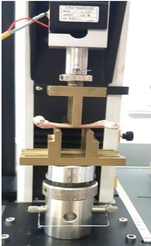
Figure [3] Rabbit femur bone in three-point bending test setup
